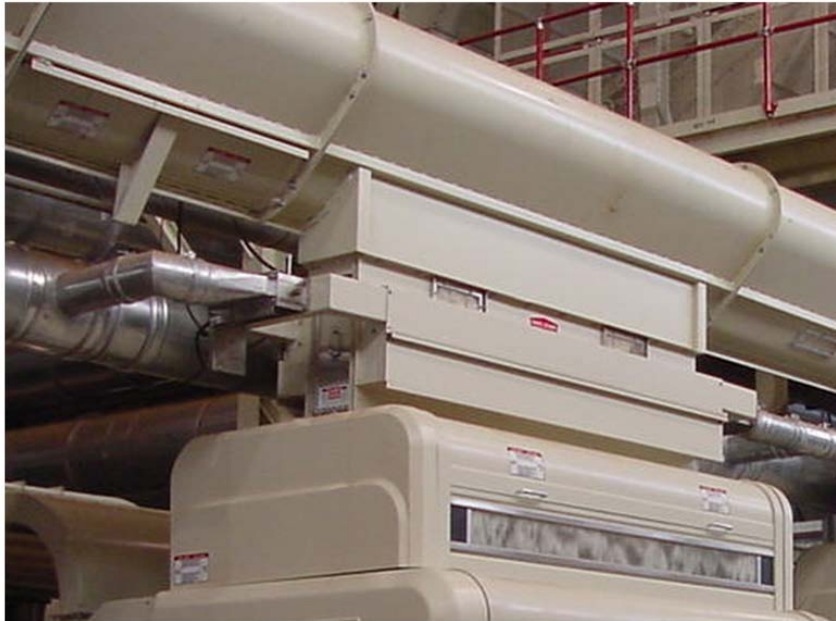
Conditioning Hopper with double air entry for high capacity gin stands (Model CH-96-1225 with moist air entry on ends shown)
