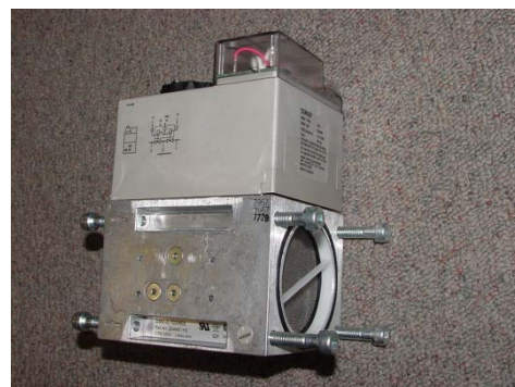
Screen on inlet to SSOV block
